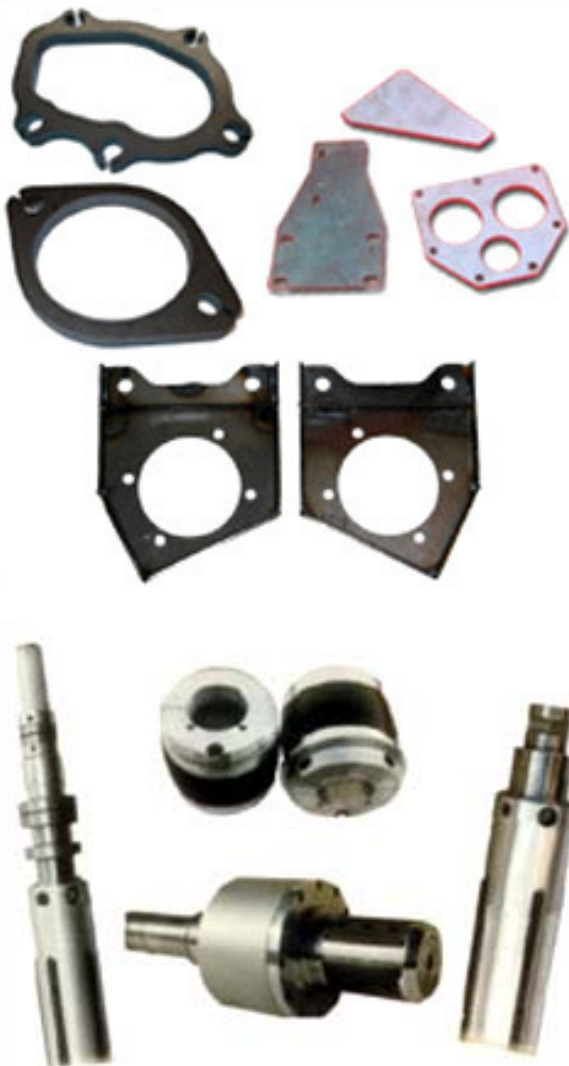
Fig.3. Engine components processed by laser cutting [2].
